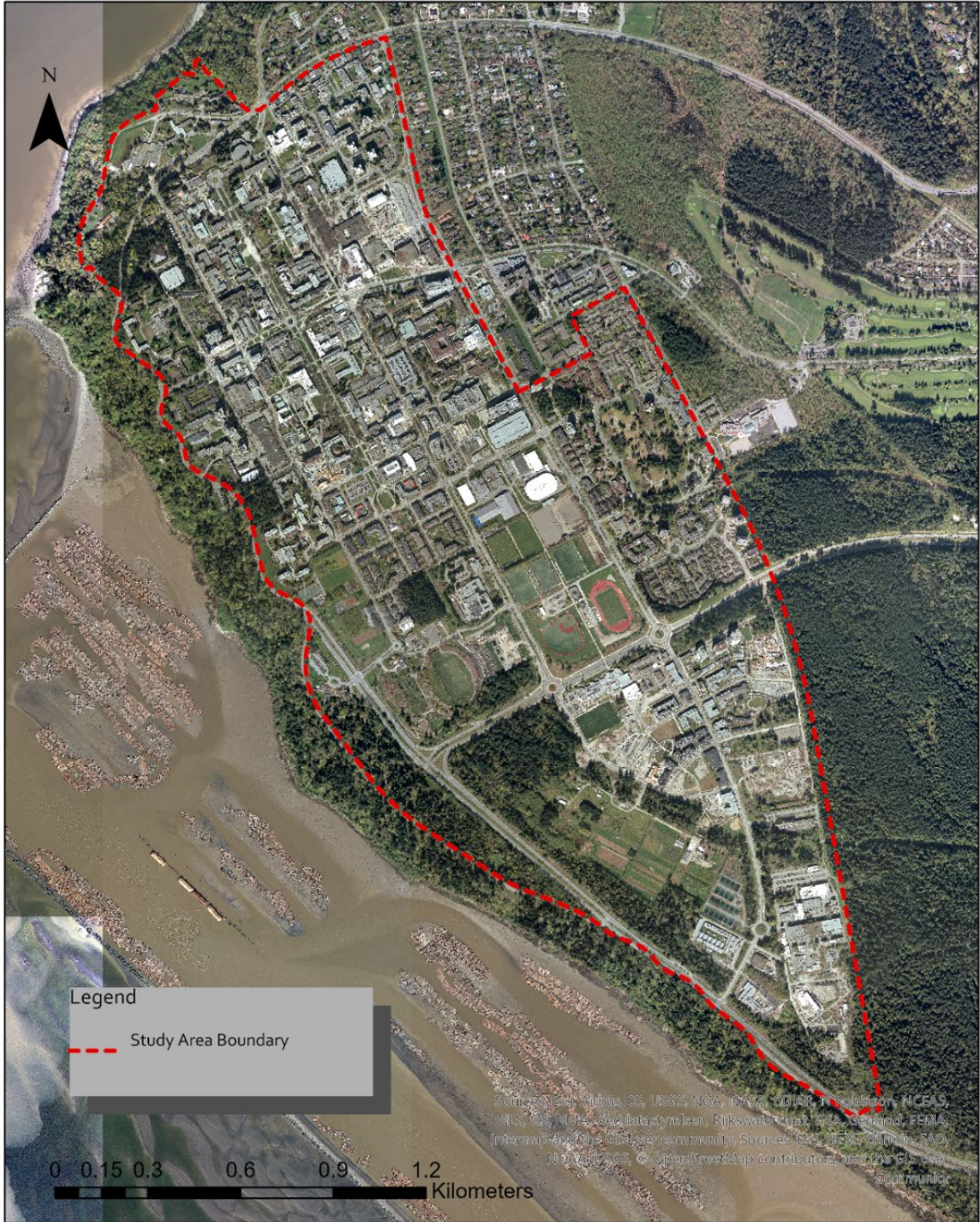
Figure 13: The map is a high spatial resolution image of the University of British Columbia Vancouver campus in 2015, with a spatial resolution of 10 cm. The map projection is NAD 1983 UTM Zone 10N. Data source: McElhanney Consulting Services Ltd., (2015). Orthophotos, University of British Columbia Vancouver Campus. Retrieved from: https://abacus.library.ubc.ca/dataset.xhtml?persistentId=hdl:11272.1/AB2/KIZZ4L .
