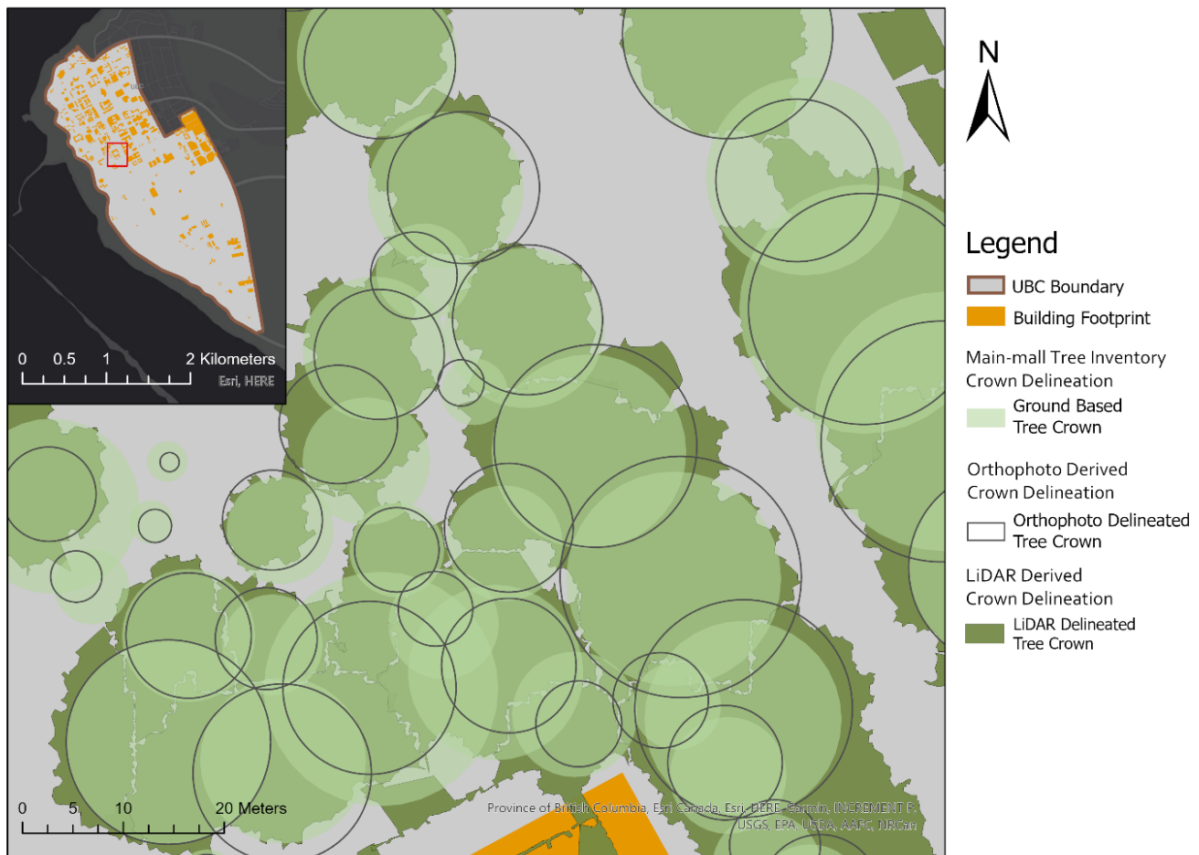
Figure 4: The subset of tree crown delineation validation in UBC Vancouver campus by the ground-based tree inventory (light green) with LiDAR (dark green) and high resolution orthophoto (10 cm spatial resolution) outlined by black circles. The map projection is NAD 1983 UTM Zone 10N.
